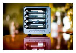
**PROS** — **security, scalability, accessibility.** The great thing about a RAID tower is that it protects itself against most hard drive failures. If one drive fails, pull it out, put a fresh one in, and let it rebuild your data. You can also upgrade your drives for additional space as the need arises. Most towers are also geared to attach to a network, so you can access them from several computers through a router.
